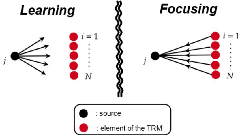
Figure 1: Learning and focusing steps of TR focusing between a source  $j$  and a TRM of  $N$  transceivers.
