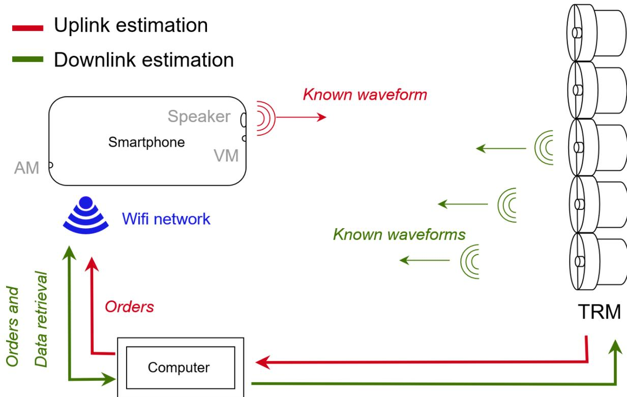
Figure 4: Bidirectional and unidirectional estimations of the propagation channel between a smartphone and a TRM.
