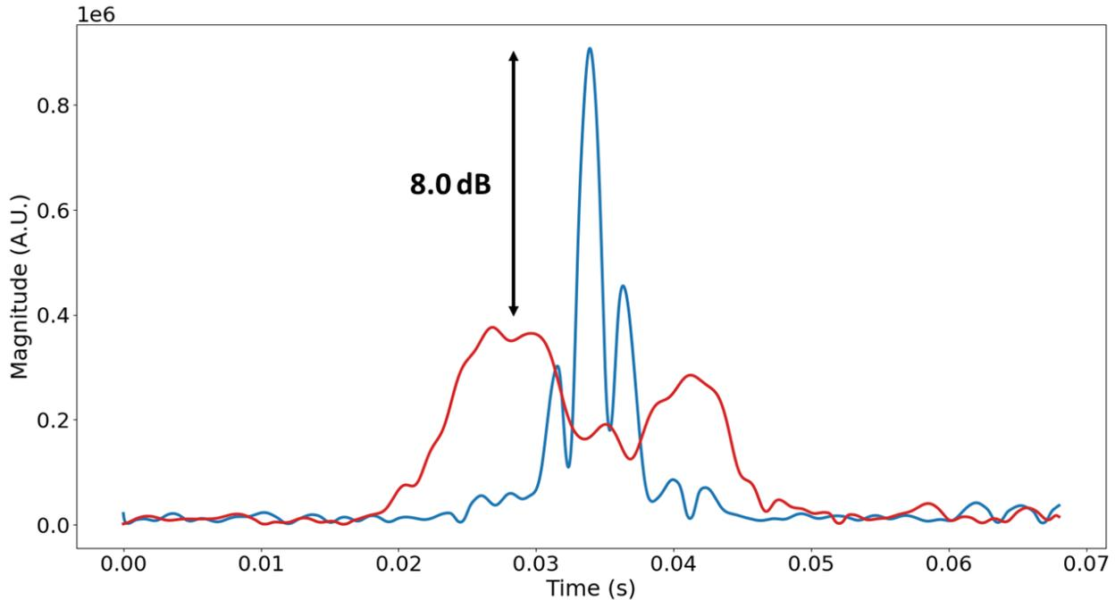
Figure 10: Envelopes of  $C_{>}(t)$  (blue curve) and  $C_{<}(t)$  (red curve) for a symbol transmission between the TRM and the VM in the case of configuration E. The symbol is focused using the UCE.
