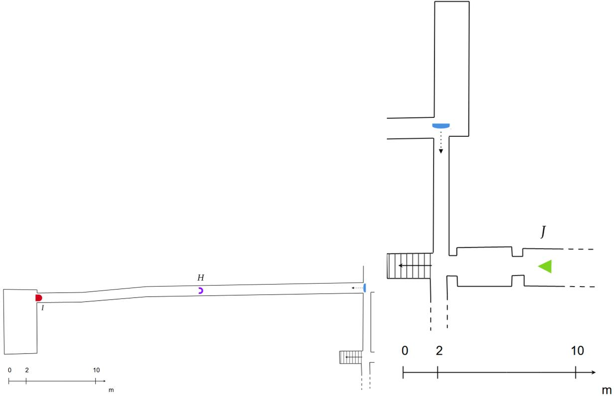
Figure 9: Left: LOS configurations in a basement between a TRM (half blue ellipse) and a smartphone (red half-ellipse and purple arc). Right: NLOS configuration in a basement between a TRM (half blue ellipse) and a smartphone (green triangle).
