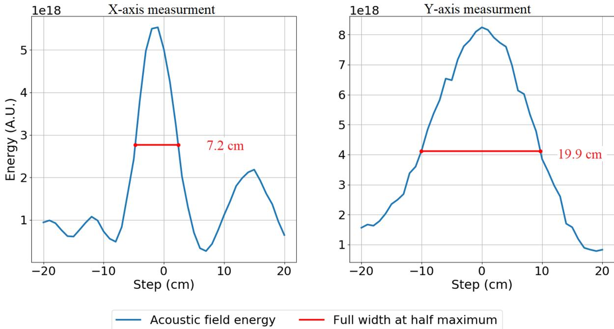
Figure 5: Focusing on a ME that is at 1.72 m from the TRM and  $16^\circ$  off-axis. Experimental focal spot over an axis parallel (on the left) and perpendicular (on the right) to the TRM.
