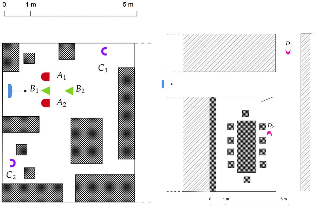
Figure 6: Left : LOS configurations in a room between a TRM (half blue ellipse) and MEs pairs (red half-ellipses, green triangles, and purple arcs). Right: NLOS configuration in a corridor and a library, between a TRM (half blue ellipse) and a MEs pair (pink crescents).
