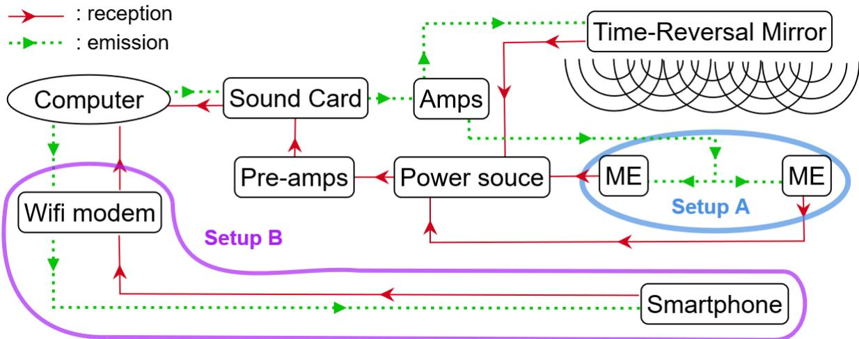
Figure 3: Acquisition chains for the setups A and B.
