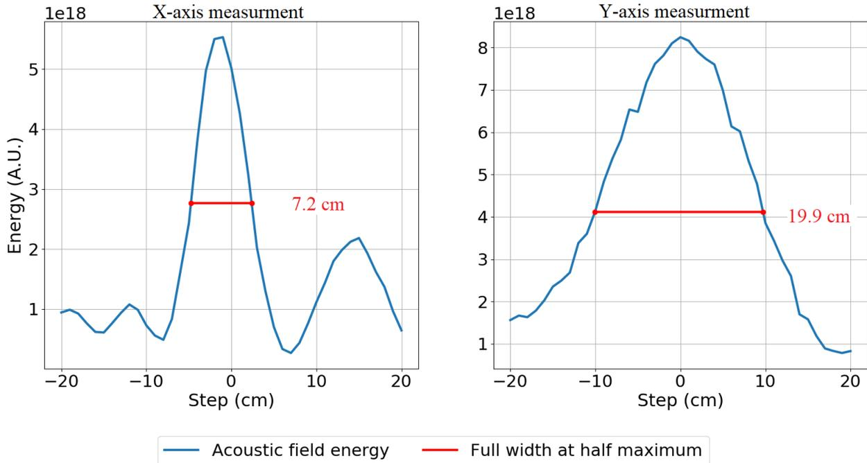
Figure 5: Focusing on a ME that is at 1.72 m from the TRM and  $16^\circ$  off-axis. Experimental focal spot over an axis parallel (on the left) and perpendicular (on the right) to the TRM.
