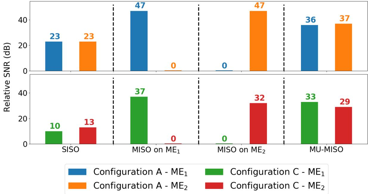
Figure 7: Relative SNRs - obtained with a single emitter, a TRM focusing successively or simultaneously on two users - for configurations A and C. The transmission power is held constant.
