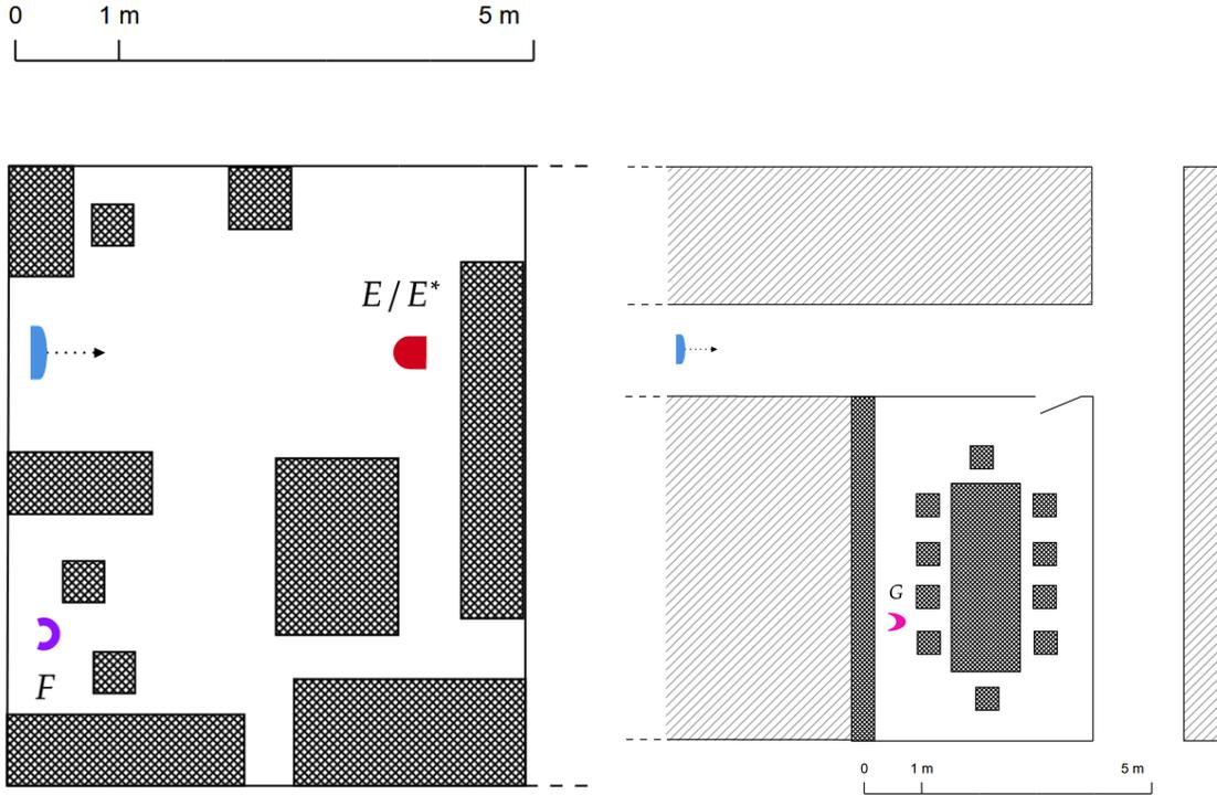
Figure 8: Left: LOS configurations in a closed rooms between a TRM (blue half ellipse) and a smartphone (red half-ellipse and purple arc). Right: NLOS configuration in a corridor and a library between a TRM (blue half ellipse) and a smartphone (pink crescent).
